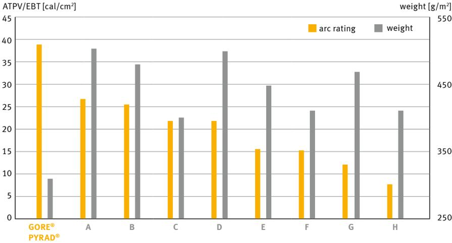
Arc rated GORE® PYRAD® garments are up to 50% lighter than other garments with class 2 arc protection. At the same time they provide the best arc rating.
